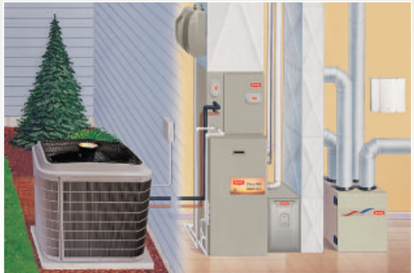
Air Conditioner and Gas Furnace System
